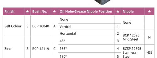
\*When ordering, please add the above 'characters' to the part number to indicate required condition, e.g. BCP11026SA1N indicates self colour with BCP10040 bush, vertical oil hole and BCP12595 mild steel grease nipple.
